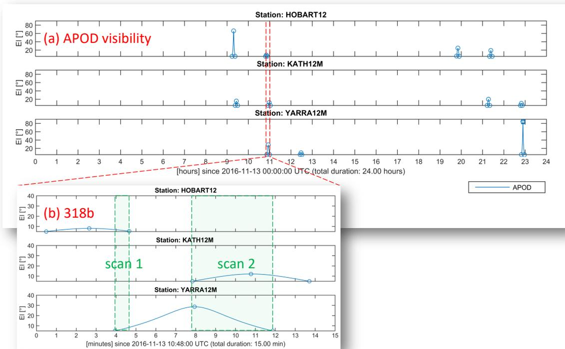
**Fig. 2** Graphical illustration of the APOD visibilities in VieVS (satellite elevation at stations versus time). After checking (a) APOD visibility roughly for the whole day (Nov. 12, 2016) and selecting suitable passes, (b) definite scan times were accurately determined. Scan durations for common visibilities are a few minutes at most.
