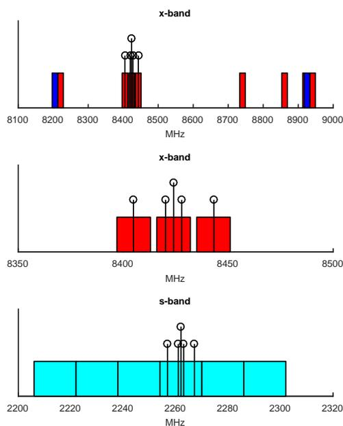
**Fig. 3** Observing mode in APOD experiments 316 to 333. We observed 16 channels with 16 MHz bandwidth at two-bit sampling. In X-band, the DOR tones are covered by channels 2 to 4 with the carrier at 8424.04 MHz. In S-band, all satellite tones lie within one channel. Due to RFI, all S-band channels were allocated contiguous to cover a continuous band.
